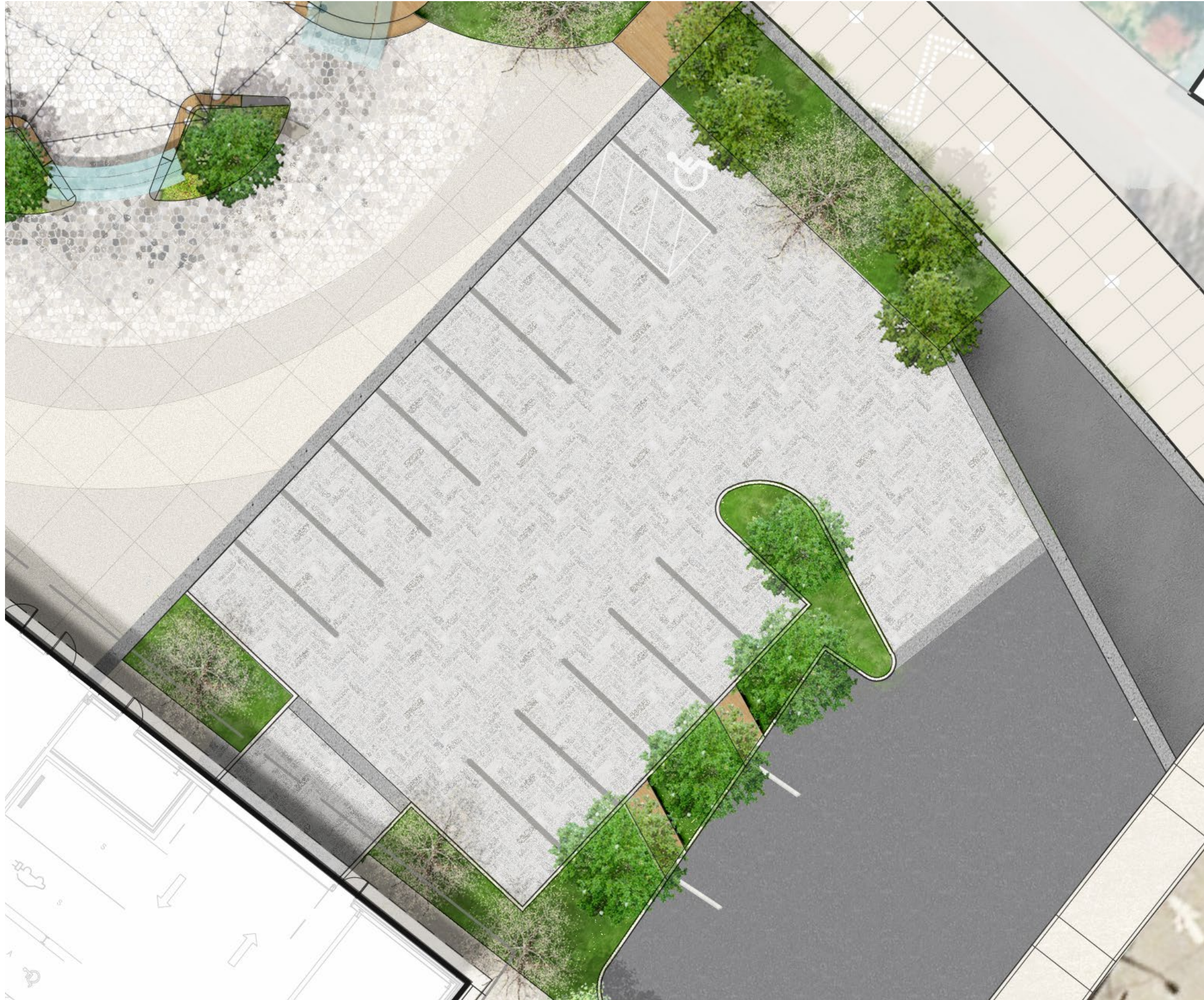
bioretention area to help capture stormwater
